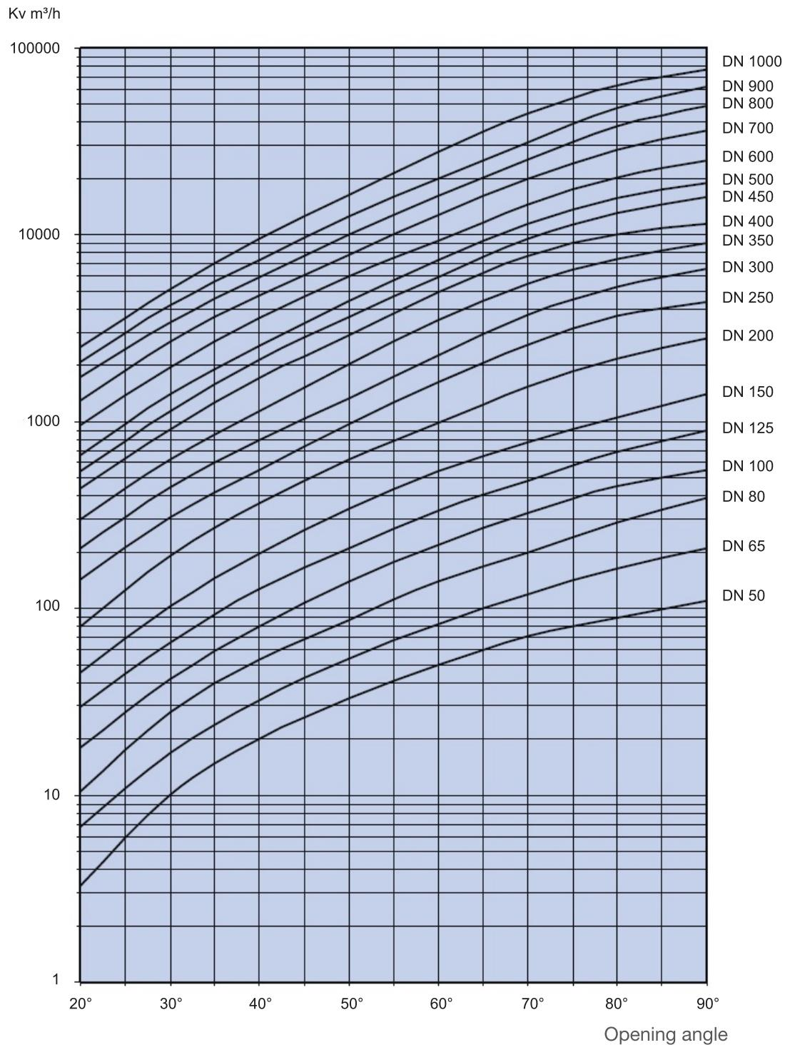
Kv = Capacity, water m³/h. T = 20°C and Δp = 1 bar
