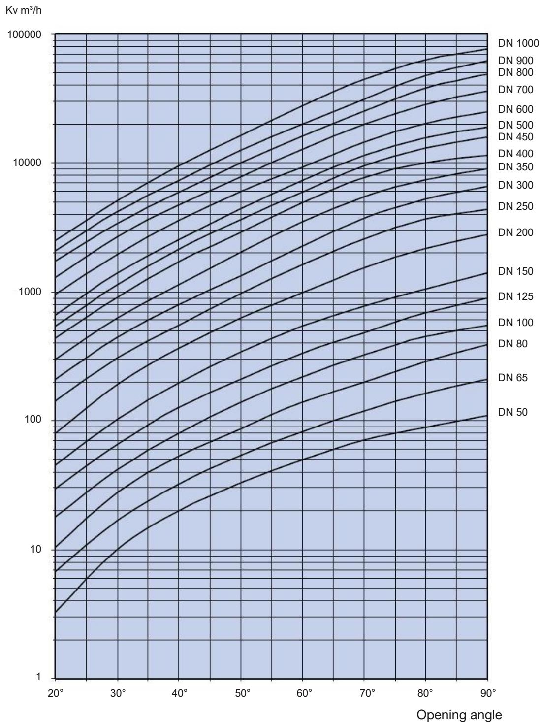
Kv = Capacity, water m<sup>3</sup>/h. T = 20°C and Δp = 1 bar
